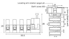
On CFTBN/1 spigot to mounting hole = 10mm
