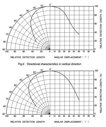
Fig.10 Directional characteristics in horizontal direction
