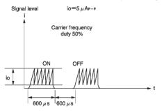
Fig.3 Standard photodiode current
