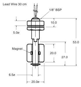
Float position can be reversed to give contacts open or closed in liquid
