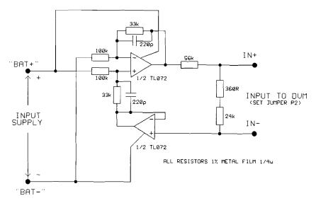
CIRCUIT TO READ INPUT SUPPLY ON PM-438
