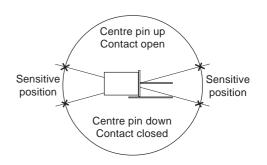
Contact Form/Style: Switch types CW1300 may have a normally open or closed contact depending on the positioning of the switch. These switches have a change in sensitivity depending on the switch position.
